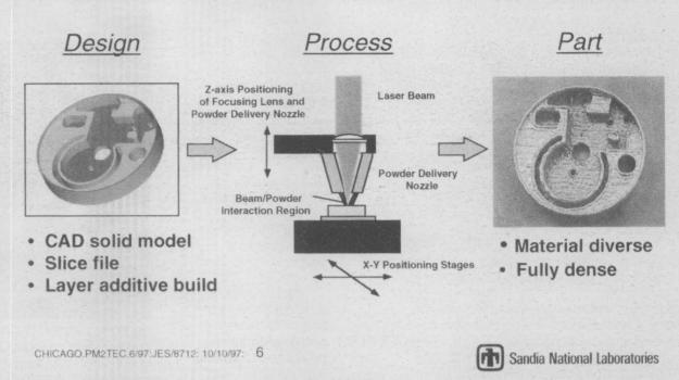
LENS fabrication converts a virtual component, such as this proposed stronglink housing, left, to an actual part, right, through building a net shape line by line and layer by layer.
